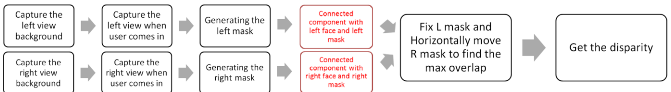
Figure3. The whole algorithm flow of refined mask based stereo matching (MBSM). The red blocks is the difference between refined MBSM and original MBSM proposed in [8].
